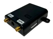
CellBox is a simple, high-value, low-cost, fully certified cellular modem terminal. Featuring LTE M1, NB1/NB2 cellular connectivity with fallback to EGPRS and a high-quality GPS receiver, CellBox lets you add cellular and GPS capability to any system with zero certification requirements.
