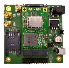
This product is a low cost LTE cellular M1 radio with support circuitry mounted on a mini-PCle carrier card. It is an FCC, ISED & PTCRB certified module, allowing for direct and immediate use in most end products with no further certification.
